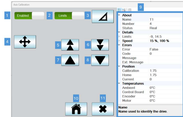
FIGURE 55 – T1 AXIS CONTROL SCREEN
