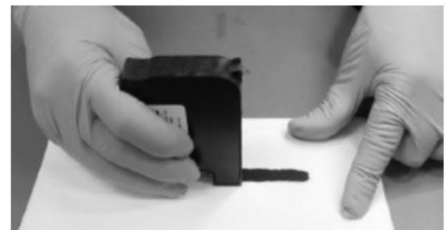
FIGURE 141 "WICKING WIPE" TECHNIQUE FOR REMOVING HARDENED DEPOSITS OF INK AND DEBRIS (LATER WIPE)
