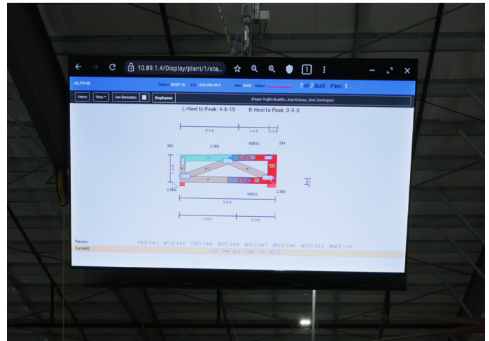
The SmartView system is an optional overhead display for real-time guidance.
