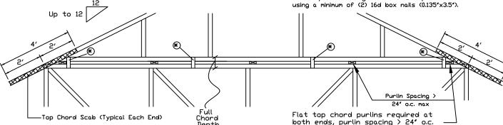
Note: If purlins or sheathing are not specified on the flat top of the base truss, purlins must be installed at 24" o.c. max. and use Detail A.
