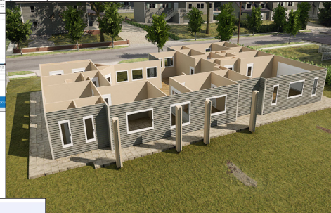
STITCHER converts 2D plan into a buildable 3D geometry
