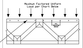
For single top chord, see chart below for screw spacing. For double top chord the screw spacing may be doubled (but may not exceed 24" o.c. per chord). Screw spacing shall be offset by 1/2 the o.c. spacing in each chord.
