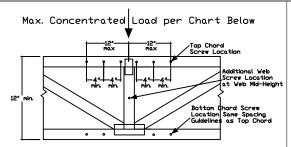
Apply screws to chords within 12" of the concentrated load location @ 4" o.c., min, evenly distributing them to each side of the concentrated load. A maximum of 6 screws may be applied to the top chord for each concentrated load.
