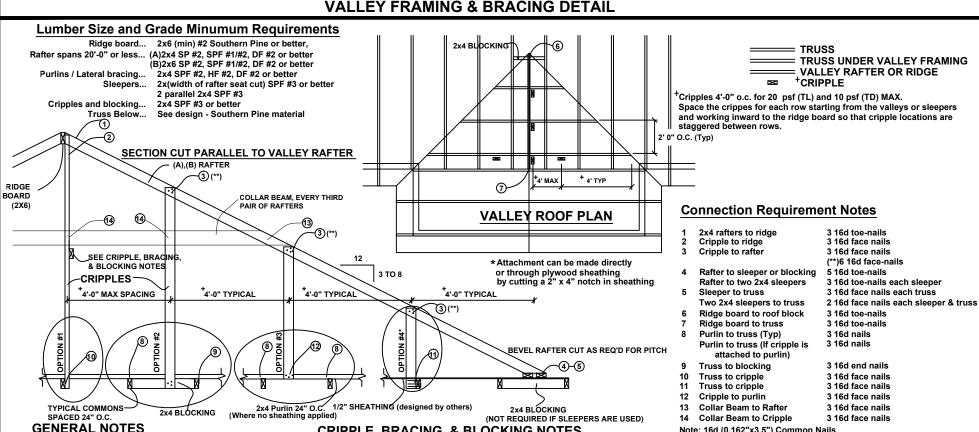
Purlins required 2'-0" O.C. in absence of plywood sheathing. Trusses without sheathing applied must be evaluated accordingly. Purlins should overlap sheathing one truss spacing minimum. In cases that this is impractical, overlap sheathing a minimum of 6". and nail upwards through sheathing into purlin with a minimum of 8-8d (0.131"x2.5") common nails. Effects of not providing sheathing below a valley set must be evaluated by the building designer.
