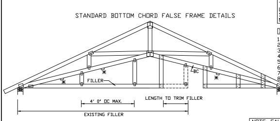
THIS DETAIL APPLIES TO ANY PITCH, ANY SPAN, ANY TOP CHORD LOADING AND ANY TRUSS WEB CONFIGURATION FOR 24" D.C. MAX. SPACING AND 10PSF MAX. CEILING LOAD, WITH THE EXCEPTIONS NOTED ON THIS SHEET
