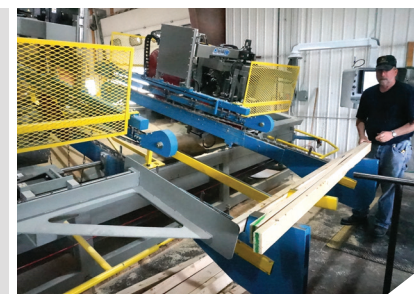
The infeed conveyor is set at waist height for enhanced ergonomics and worker safety.
