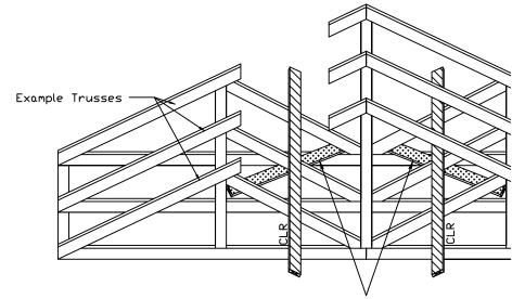
2x4 diagonal bracing nailed to opposite face of web and repeated at approximately 20 foot intervals to resist lateral movement. Attach to webs with (2)-10d (0.128"x3.0",min) nails. Diagonal bracing may traverse more than two trusses, depending on truss height.
