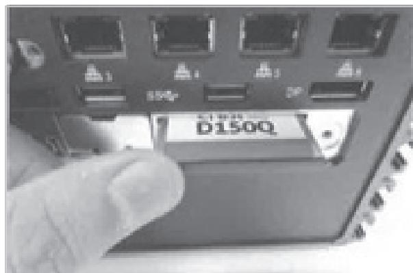
Replace cover after inserting the new C-Fast card.
