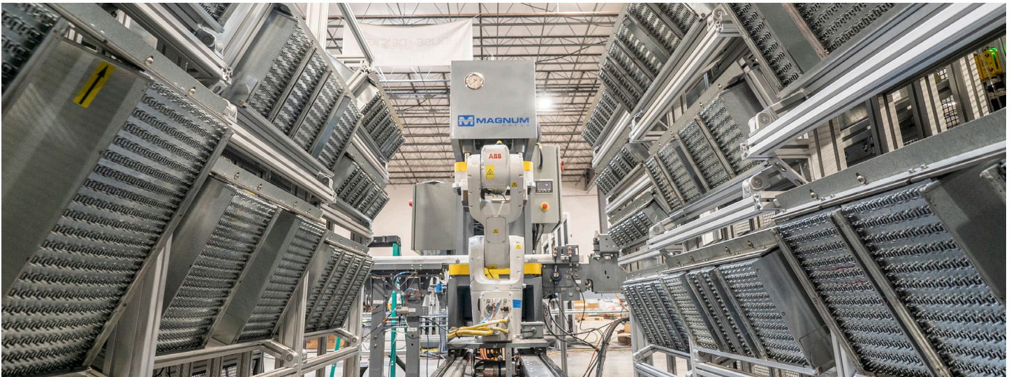
House of Design's preplate station—preplating members for robotic assembly. A key to reducing safety hazards and pick errors.
