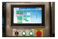
The Ranger has its own control panel that is used for startup and trouble shooting. During production, all Ranger functions are controlled by the ALS 4.0 Linear Saw.
