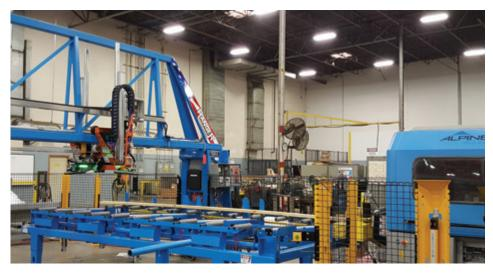
The Ranger loads an infeed designed specifically for the Alpine ALS 4.0. The Ranger automatically picks and places the board onto the infeed guaranteeing correctly sized boards enter the saw in the right order.
