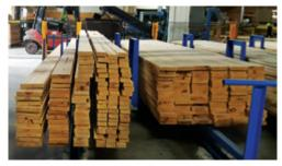
Two types of carts are available with the Ranger. Lumber carts hold a full bunk of lumber and are sloped for lumber stability during picking. Magazine carts hold quantities of lesser used lumber and have moveable posts to customize their configuration.
