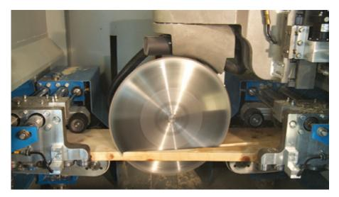
The ALS 4.0 is equipped with a 20.5 Inch blade. This allows the saw to cut all pieces, even for the most difficult trusses. Beveling models can cut bevels, double bevels and ripped valley bottoms.
